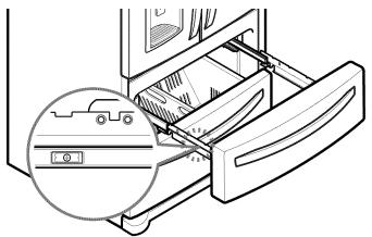
**3.** With both hands, hold both sides of the door and pull it up to separate it from the rails.
